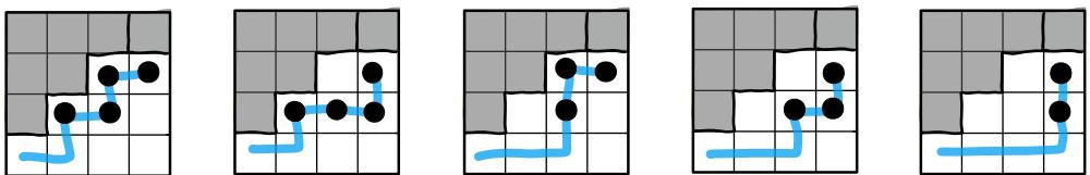
Process multiple dots in sequence as encountered, depth first search
